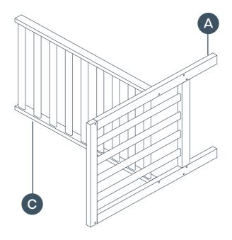
Clear an area on the floor and lay the mattress slat base (C) and cot end (A) on their sides, being careful not to scratch the frame.
